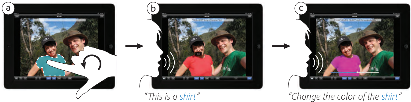
Figure 1. With PIXELTONE, users speak to edit their images instead of hunting through menus. a) The user selects the person’s shirt and says “This is a shirt.” PIXELTONE associates the tag “shirt” with the selected region. b) The user tells PIXELTONE to “Change the color of the shirt,” and c) PIXELTONE applies a hue adjustment to the image and offers a slider so that the user can explore different colors.
